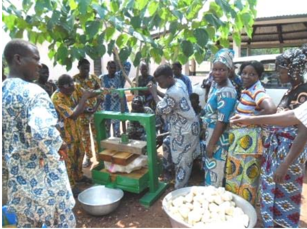
Yam bean BE Group 1 INRAB Photo 26: Screw press and yam bean pressing demonstration for juice extraction at on-farm scale at Dangbo (South Benin) (photo by W. Padonou, 2013).
