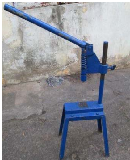
Yam bean BE Group 1 INRAB Photo 16: Manual bottle capper fabricated by INRAB to cover bottles filled with yam bean juice (photo by W. Padonou 2013).
