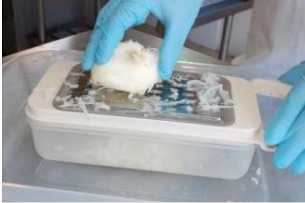
Yam bean PE Group 4 Photo 17: During ahipa root laboratory processing, ahipa roots without their skin are grated on a stainless steel grater to determine plant iron and zinc of processed ahipa products without non-plant iron and zinc contamination (photo by research assistant R. Carpio, 2012).
