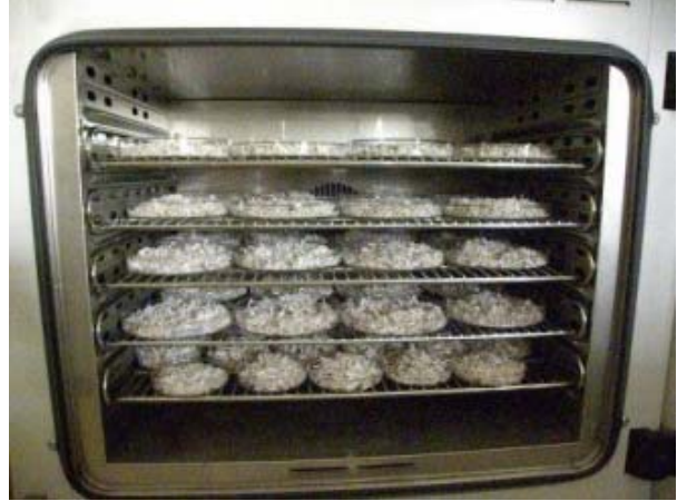
Yam bean PE Group 4 Photo 22: Drying of the wet ahipa cake. It shows the broken wet cake in small pieces (grits), placed in petri plates, and then put in drying oven to determine plant iron and zinc of processed ahipa products without non-plant iron and zinc contamination (photo by research assistant R. Carpio, 2012).
