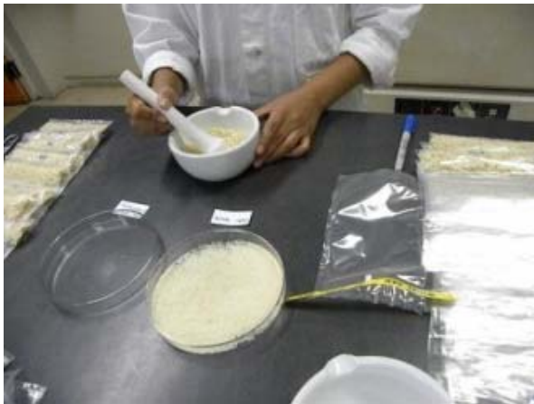
Yam bean PE Group 4 Photo 23: Milling of yam bean gari , showing the harder particles being ground with a pestle and mortar. The grits had to be milled to a specific size. Processing was conducted under conditions avoiding non-plant iron and zinc contamination (photo by Ing. C. Tasso, 2012).
