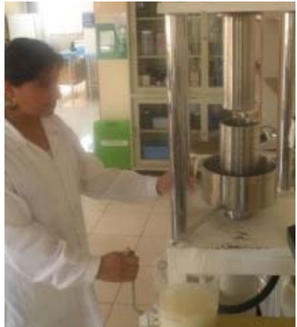
Yam bean PE Group 4 Photo 20: During the dewatering mash into wet cake, ahipa mash is pressed in the hydraulic press to remove excess water in order to determine plant iron and zinc of processed ahipa products without non-plant iron and zinc contamination (photo by Ing. C. Tasso, 2012).
