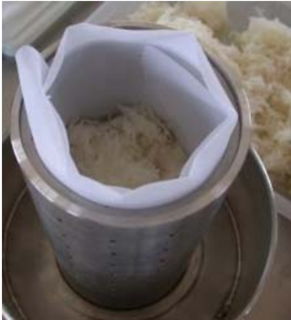
Yam bean PE Group 4 Photo 19: During the ahipa mash preparation for dewatering, a researcher puts the sample in a cotton mesh and then into a stainless steel cylinder with holes drilled to determine plant iron and zinc of processed ahipa products without non-plant iron and zinc contamination (photo by research assistant R. Carpio, 2012).
