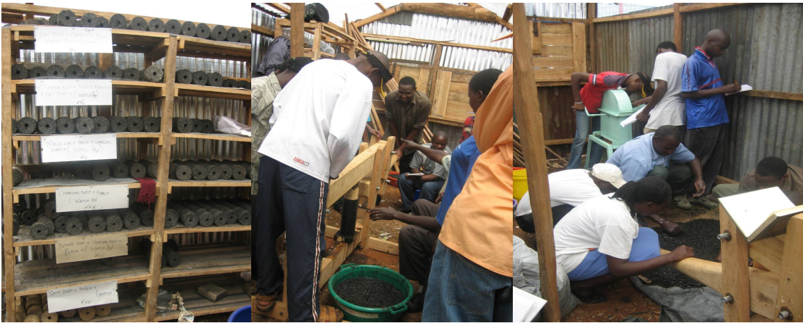
Plate 2. Drying rack, wooden press and paper shredder set up at SOYIA briquette processing plant, Kahawa Soweto.
