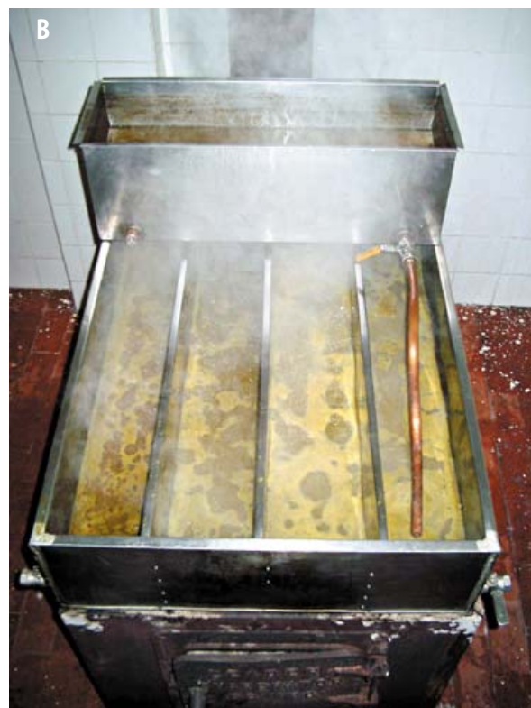
Figure 16. Evaporator. A. Complete view of evaporator: furnace, evaporation tray, reception tank and chimney. B. The evaporator in operation.
