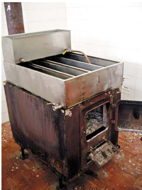
Figure 16. Evaporator. A. Complete view of evaporator: furnace, evaporation tray, reception tank and chimney. B. The evaporator in operation.
