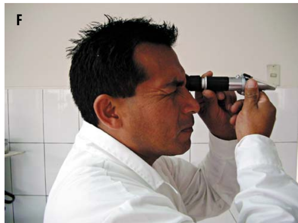
Figure 5. A quick simple method for estimating the sugar content of a lot of yacon roots. A. Randomly select a minimum of five yacon roots and peel them. B. Cut a central slice 1 cm thick from each root selected. C. Divide each slice into several pieces. D. Remove the juice with the help of a lime squeezer. E. Place a couple of drops of the juice on the prism of a portable refractometer. F. Take the reading. The value measured (in °Brix) is an estimate of the percentage of total sugars in the juice and have a high correlation with the FOS content.
