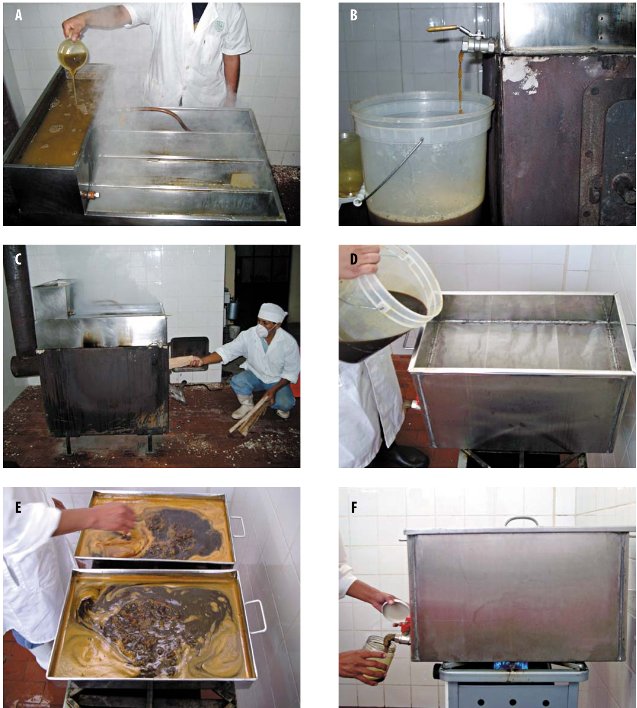
Figure 10. Different stages of processing. A. Evaporation of yacon juice. B. Obtaining the pre-syrup (50 to 60° Brix). C. Feeding blocks of firewood into the furnace. D. Filtering. E. Concentration of the pre-syrup in small trays to between 68 and 70° Brix. F. Final concentration of syrup (72 a 74° Brix) and bottling.
