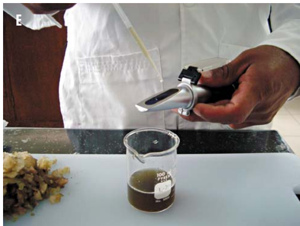
Figure 5. A quick simple method for estimating the sugar content of a lot of yacon roots. A. Randomly select a minimum of five yacon roots and peel them. B. Cut a central slice 1 cm thick from each root selected. C. Divide each slice into several pieces. D. Remove the juice with the help of a lime squeezer. E. Place a couple of drops of the juice on the prism of a portable refractometer. F. Take the reading. The value measured (in °Brix) is an estimate of the percentage of total sugars in the juice and have a high correlation with the FOS content.
