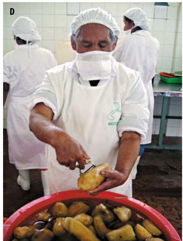
Figure 6. Peeling. A. Different models of domestic peelers which can be used to peel yacón roots. B. Details of a simple ergonomic model. C. Two women in the middle of peeling in the APYEDO processing plant (Association of Producers of Ecological Yacón and Derivatives of Oxapampa (APYEDO)), Pasco, Peru. D. Right after peeling, the roots are submerged in cold water to prevent their turning dark.
